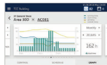
Display operating time and sensor information
